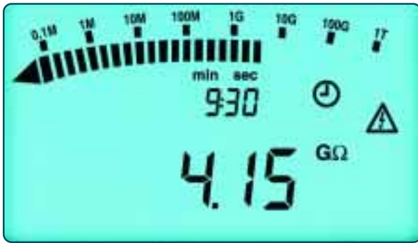
Insulation Resistance Measurement displayed throughout the test
