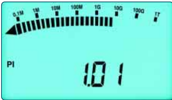
Automatic calculation and display of PI Ratio
