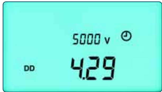
Automatic calculation and display of DD Ratio on request
