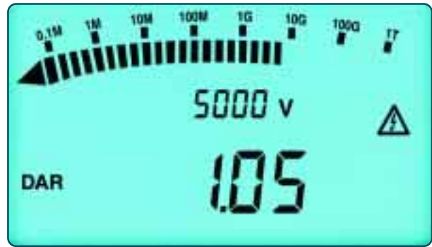
Automatic calculation and display of DAR
