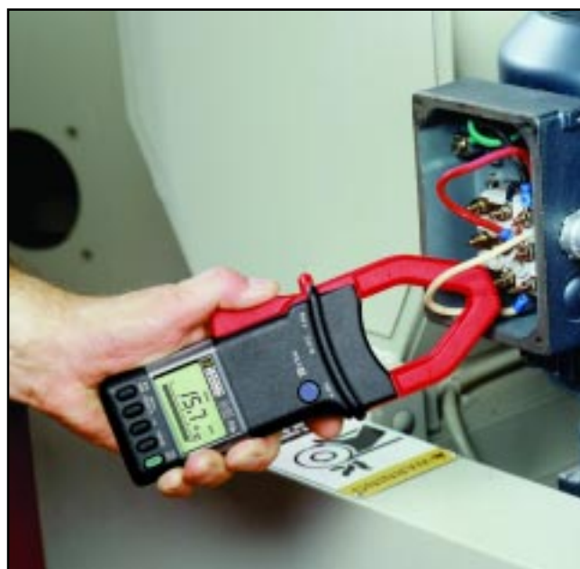
Model F3N measuring phase current on a 3 phase motor.
