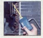
The AccuTrak VPE is compact, and designed for one hand operation. Comes with flexible wave guide for hard to reach areas.
