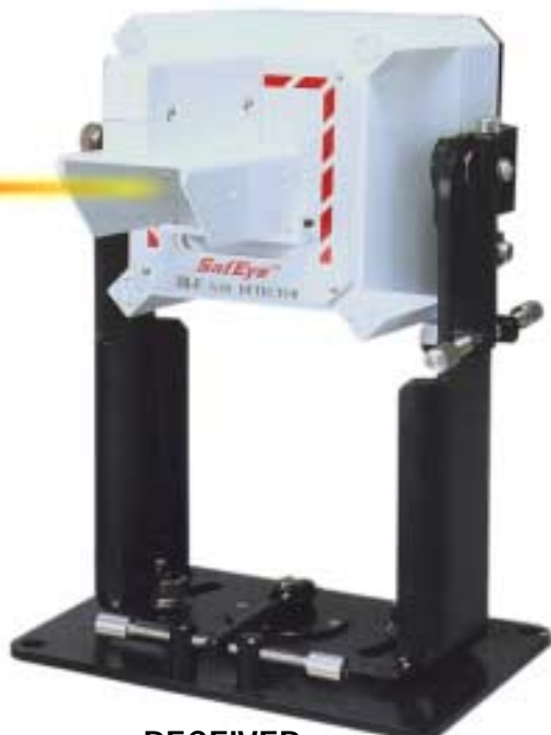
RECEIVER (Tilt mount assembly shown)
