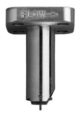
The Signet 525 Metalex Paddlewheel Flow Sensor combines stainless steel construction with insertion paddlewheel technology. The result is a highly reliable sensor suitable for operation at extreme pressures and temperatures. The Tungsten Carbide shaft and carbon fiber reinforced PTFE bearing provides excellent wear resistance for extended service.
